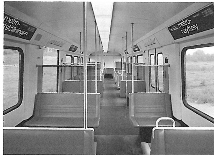
Car with cushioned seats. Fluorescent lamps along centre line of ceiling.
