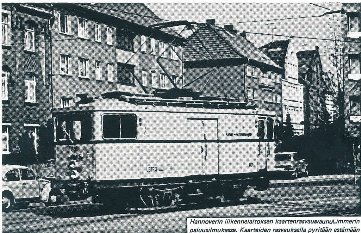
Curve-greasing car at Limmer loop in Hannover.
