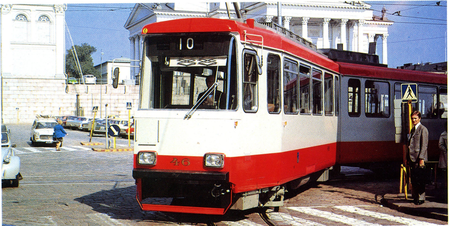
A large windscreen with wipers and washing devices and two headlights improve safety in traffic. The smallest radius of curve in the track is only 15 m.
