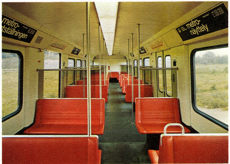
Car with cushioned seats. Fluorescent lamps along centre line of ceiling.
