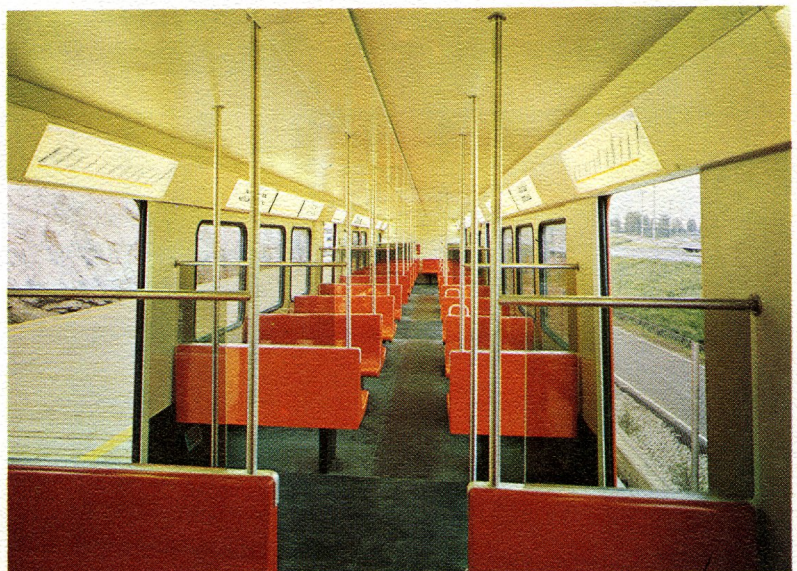
Car with seats of hard, reinforced plastics. Lamps above windows. Route maps above doors and on surface of lamps in the middle of the compartment.
